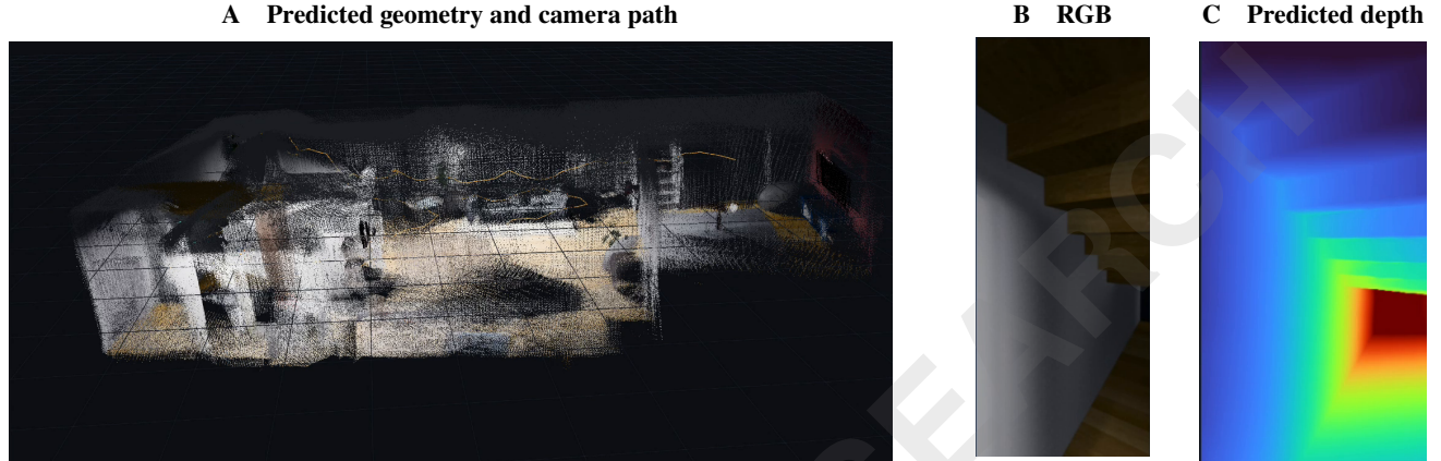
Figure 1: Single-scene prototype evidence. Crops from the supplied viewer recording at 00:00.5; image content is unchanged. The colored point display and trajectory are shown beside the selected RGB view and predicted depth. The selected preview is view_067.png ; the accumulated display contains 214 observed frames. These are qualitative model outputs, not reference geometry or accuracy measurements [1, 2].
